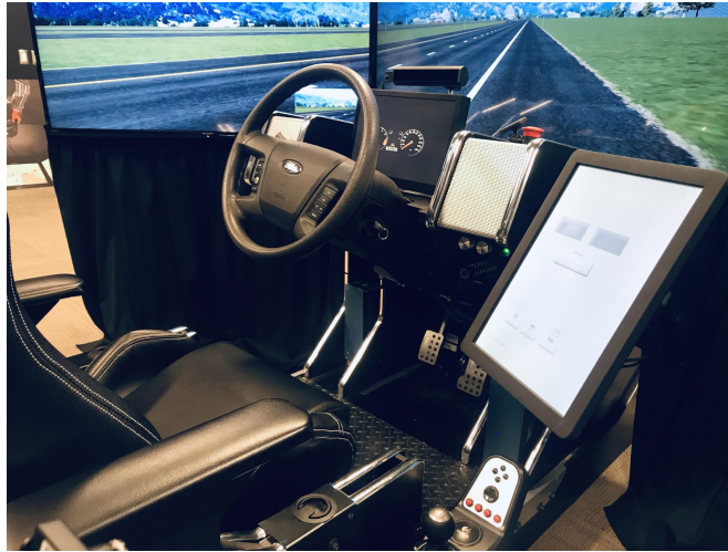
Figure 3.2 The center console with the automation activation/deactivation screen. Reprinted with permission from Alambeigi & McDonald (2021b).
