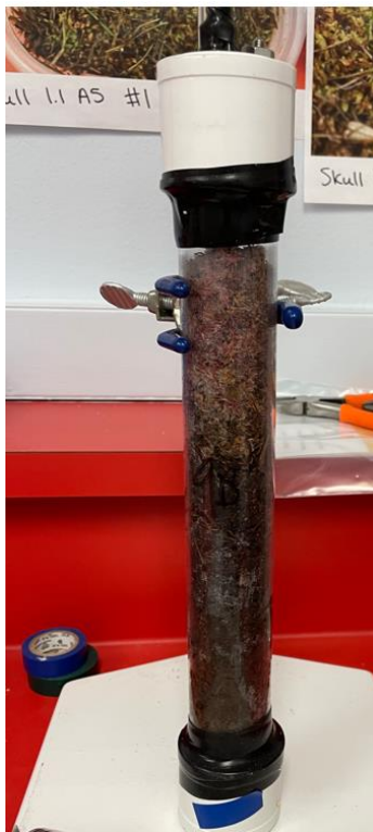
Figure 3. Image of Core 9B. This sample was a lowland peat core incubated in the 6.5C treatment. The sampling gas cap is visible attached at the top. The photo was taken directly after CO 2 sampling with the EGM-5, and the gas cap was removed once measurements were recorded and scrubbed air was injected back into the core.
