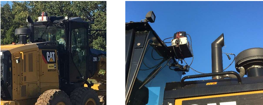
Figure 17. Motor Grader PEMS Installed
