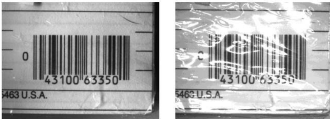
Figure 4.2. reflection effect on plastic wrapped barcode target[82].
