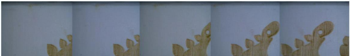
Figure 3.12. End mill tool phase-shifting raw image from location 1~5
