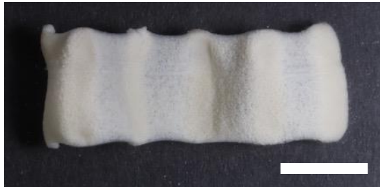
Figure A-18: Shape change of 4D printed structure in response to a second stimulus. Growth of patterned bilayer in medium containing the second biochemical stimulus for 144 h (Scale bar: 10 mm). Printed structures were first grown in synthetic medium with L-tryptophan but lacking L-leucine for 48 h (as shown in Figure 6) and then they were grown in synthetic medium with L-leucine but lacking L-tryptophan for 144 h. Bilayers were grown at 30 °C under shaking and aerobic conditions. Medium was changed every 12 h. Reprinted with permission from [296]. Copyright (2021) Wiley-VCH.
