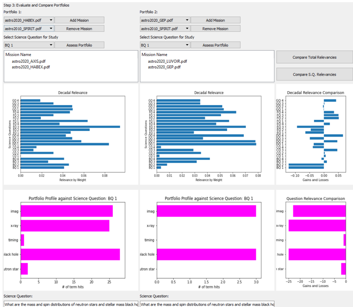
Figure 17: Region 4's relevance assessment panel. Here, the histogram plots can be viewed across two portfolios under comparison detailing the impacts these portfolios have on all/select science questions (science questions are listed via their ID number and printed after assessing the 'portfolio').
