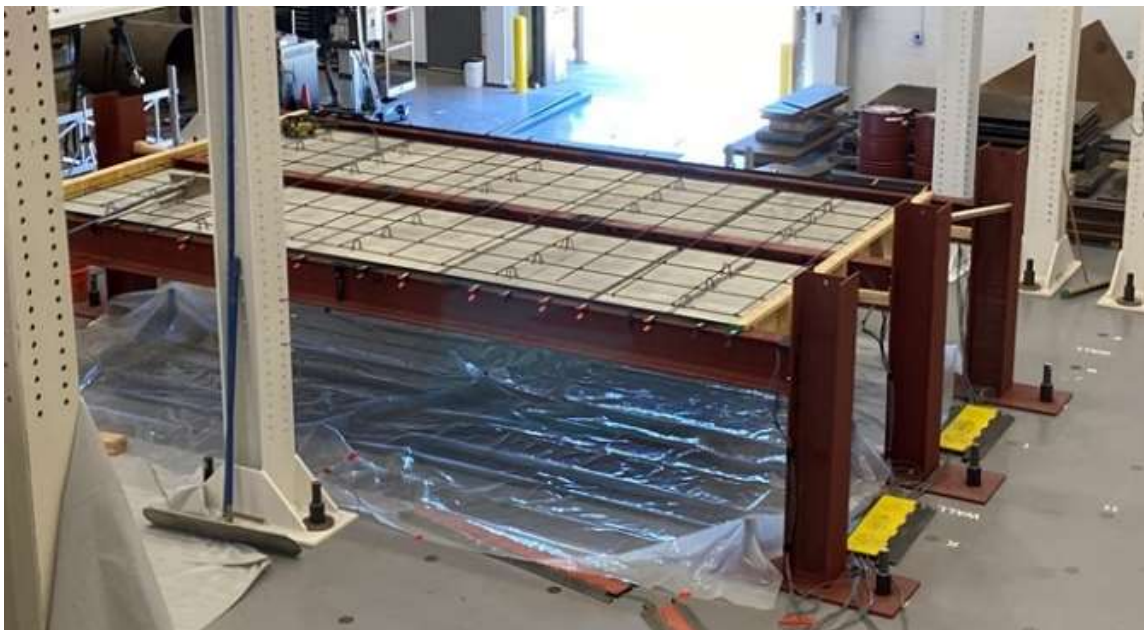
Figure 70: Concrete slab rebar reinforcement tied mat
