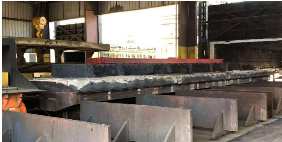
Figure 29: Reheated POC A-shape beams being removed from the oven
