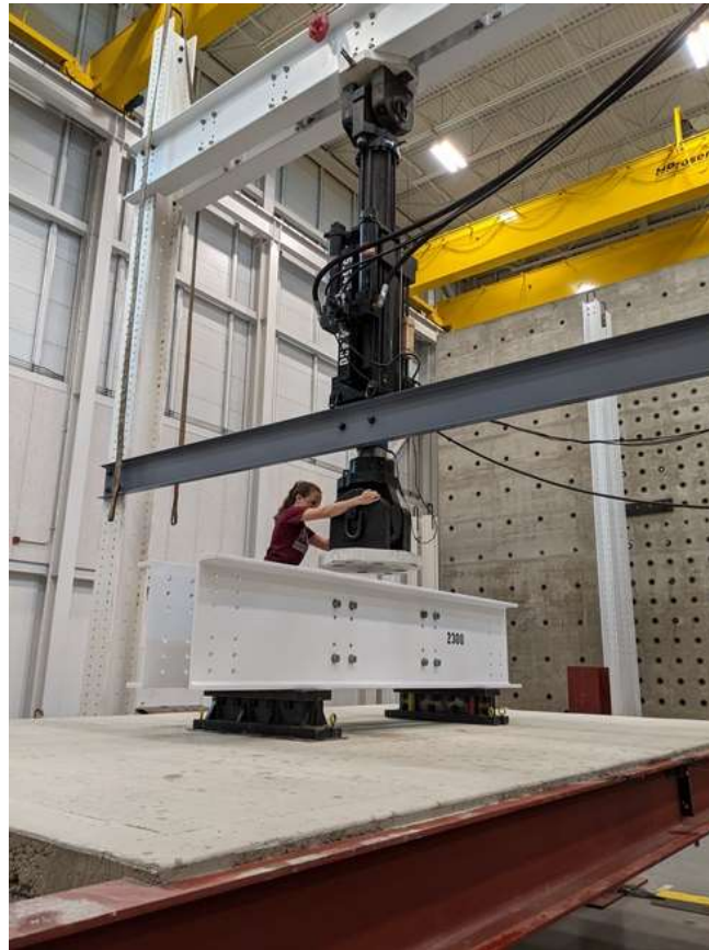
Figure 77: Spreader beam and 220 kip actuator (image by Matthew Yarnold)
