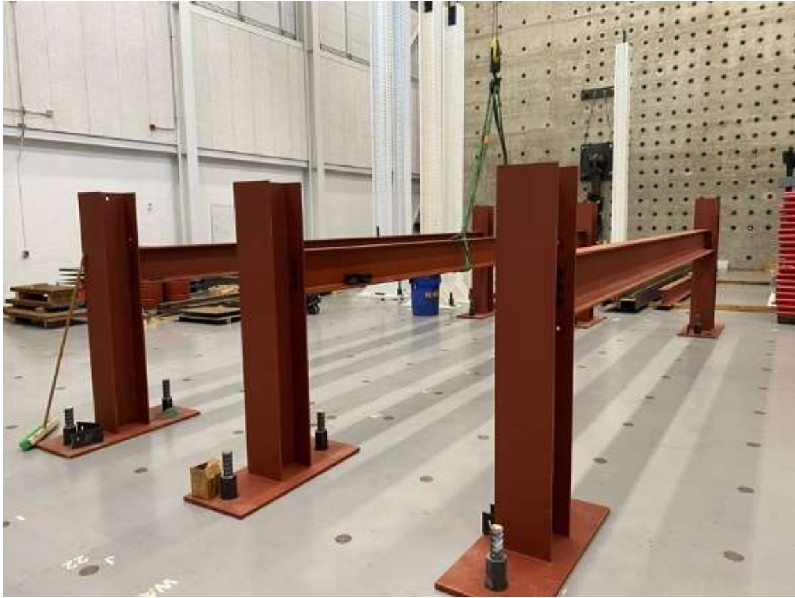
Figure 46: Floor system steel frame assembled
