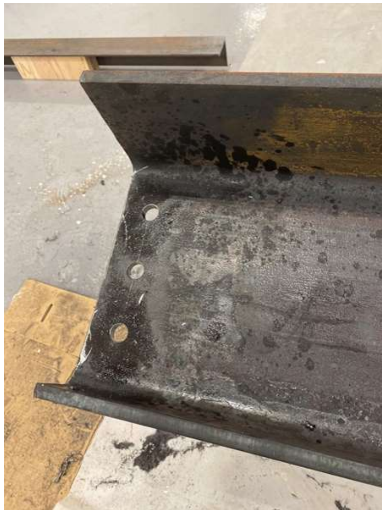
Figure 39: Center A12x53 connection holes
