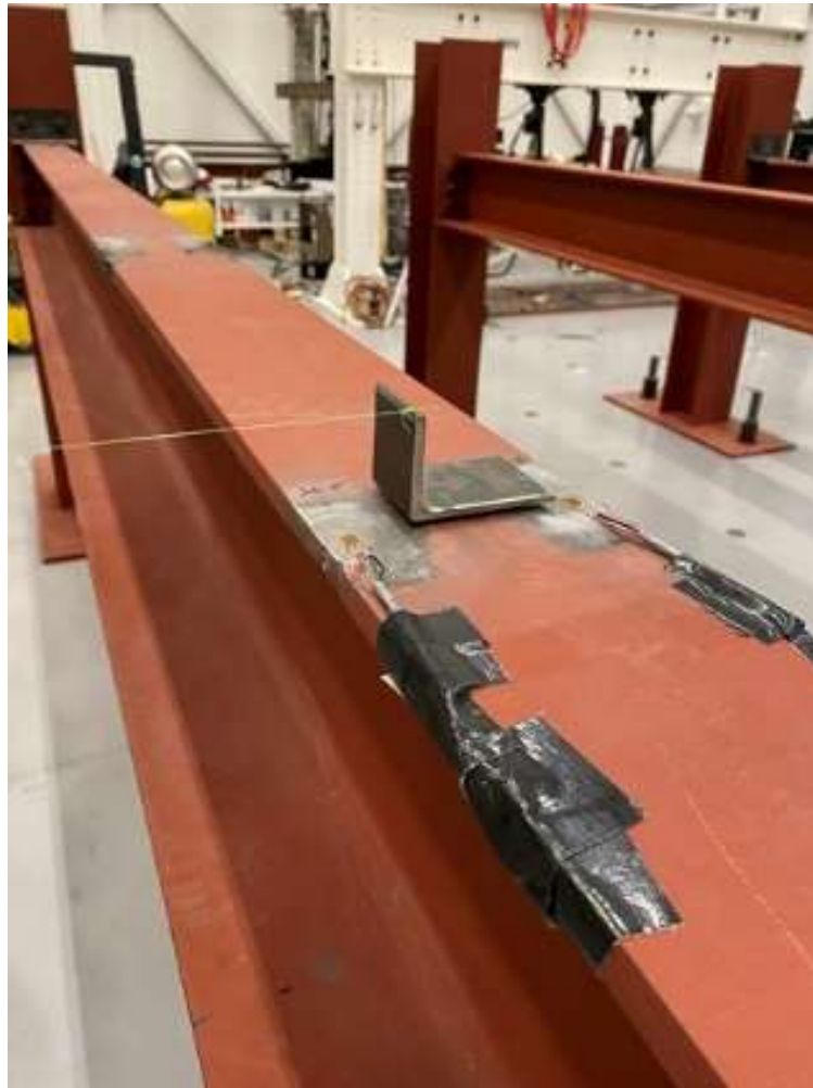
Figure 52: Edge beam top flange string-pot beam attachment
