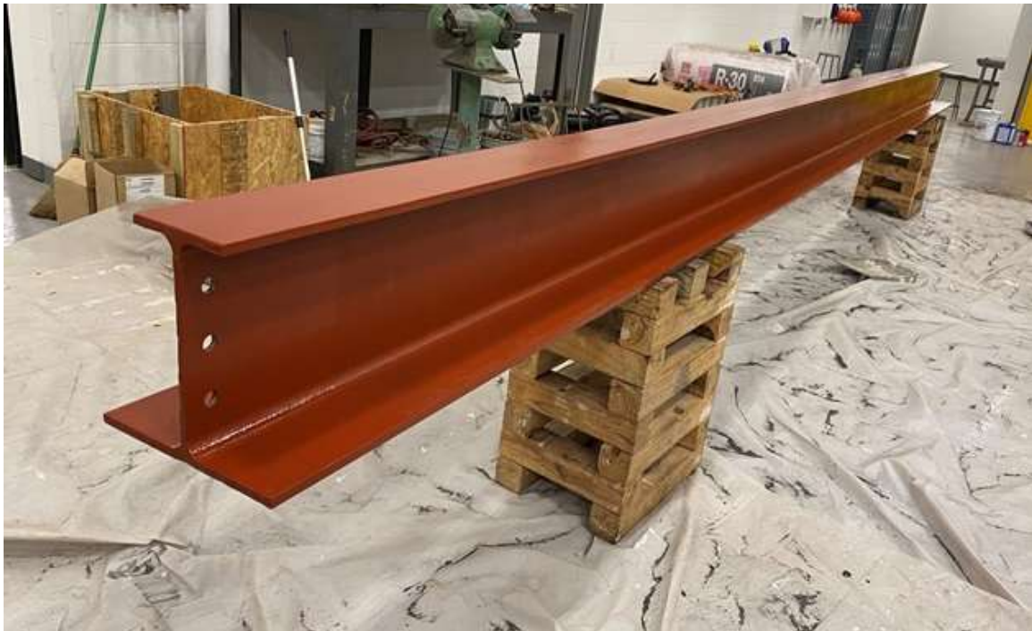
Figure 40: Center A12x53 beam primed and drilled
