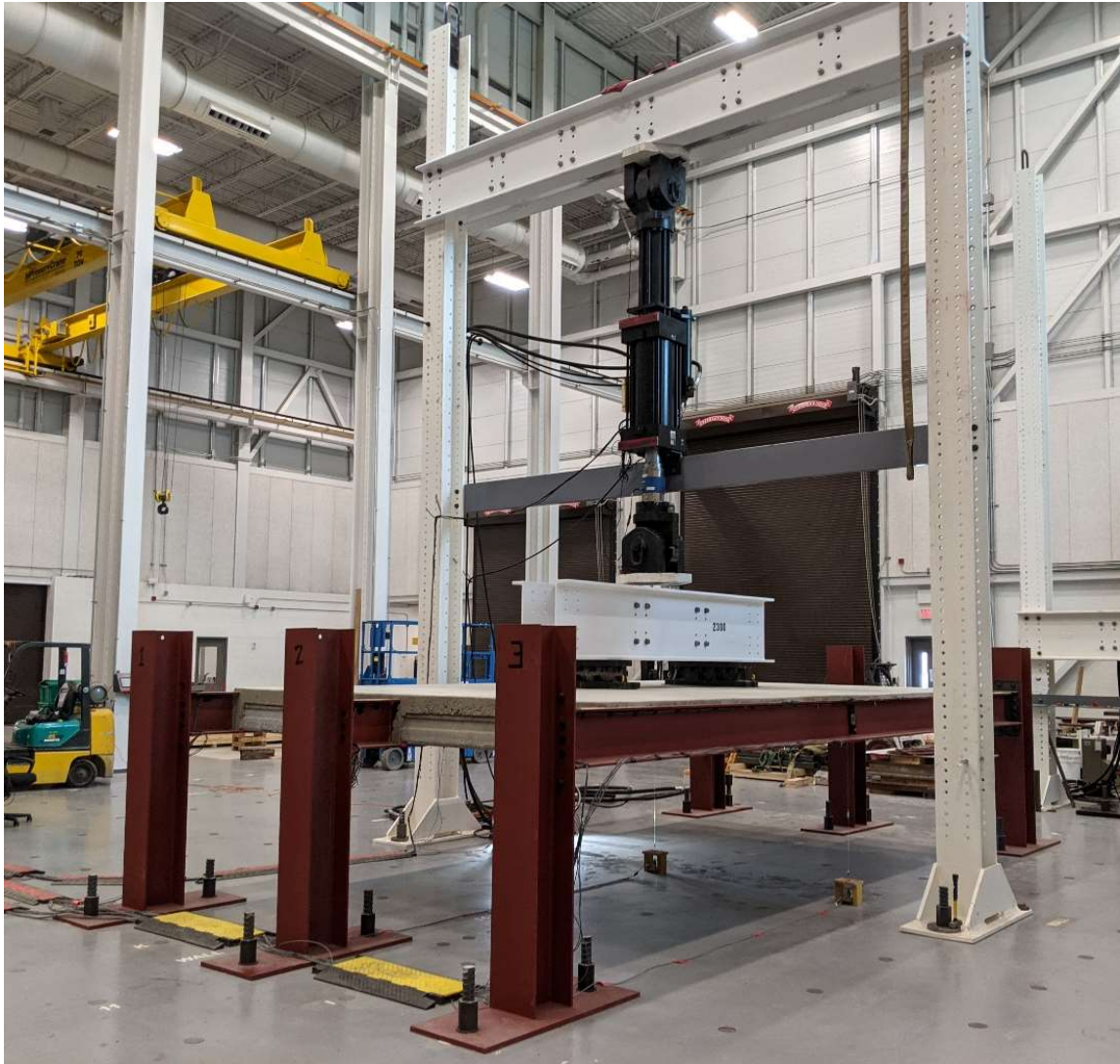
Figure 76: Floor system with loading frame and 220 kip actuator (image by Matthew Yarnold)
