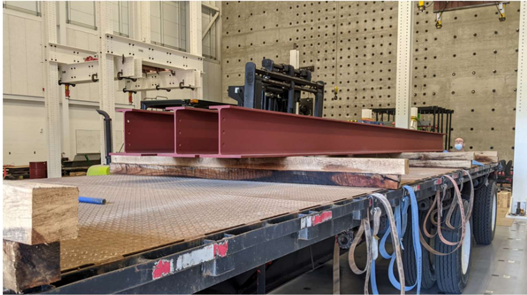
Figure 34: A12x53 fabricated A-shape beam delivery (image by Matthew Yarnold)
