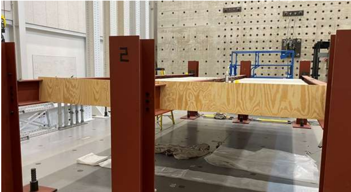
Figure 65: Floor system concrete plywood end forms
