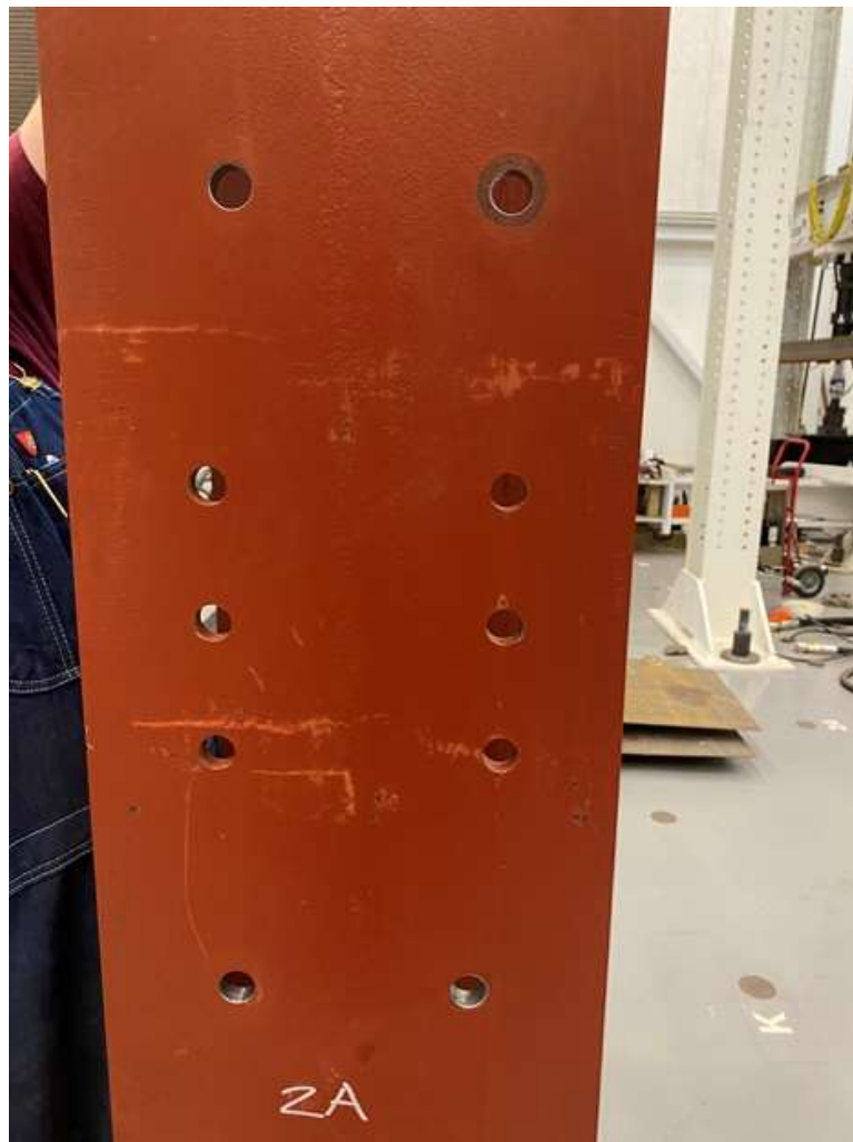
Figure 41: Edge W12x65 stub column with connection holes
