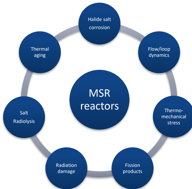
Figure 5. Summary of physical mechanisms affecting materials in MSRs.
