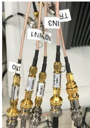
Figure 38. Proper coil attachment with limiters shown.
