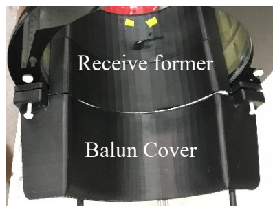
Figure 35. Proper receive coil insertion and balun cover attachment to the transmit coil.
