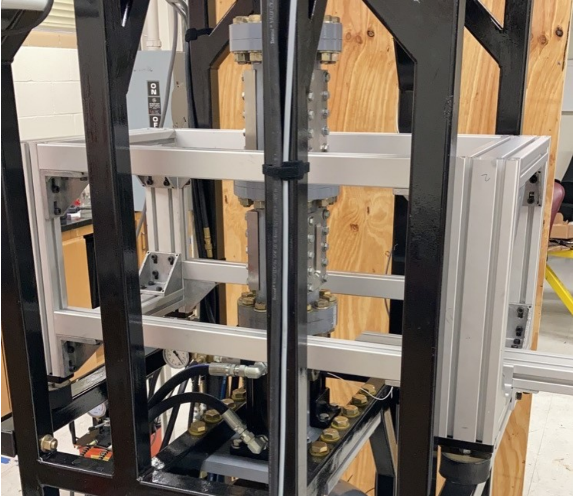
Figure 2.8: Image of mounting frame for optical diagnostics.
