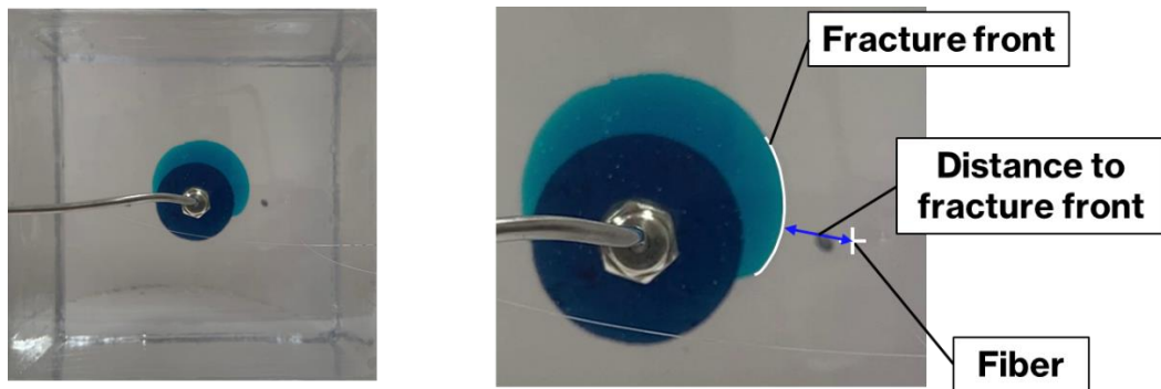
Figure 5.5 Eccentric fracture with non-radial geometry used to validate the zero strain location method
