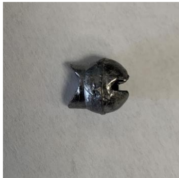
Figure 3.12 Removable split shot fishing weight used in the strain calibration procedure.
