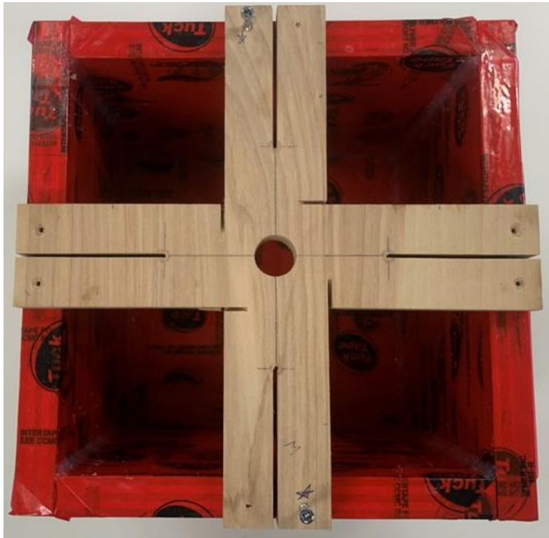
Figure 3.20 Fiber positioner assembled to the top of the epoxy mold.
