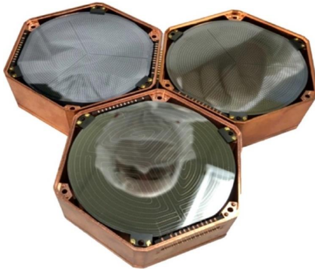
Figure 3-1 Cryogenically cooled Ge/Si detectors with photo lithographically patterned Transition Edge Sensors provide energy and position information. These detectors utilize the technology developed for the Super CDMS experiment. Each detector measures about 1.6 kg [8].
