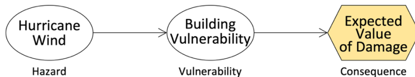
Figure 4. BN for the risk assessment of the hurricane wind on home structures.
