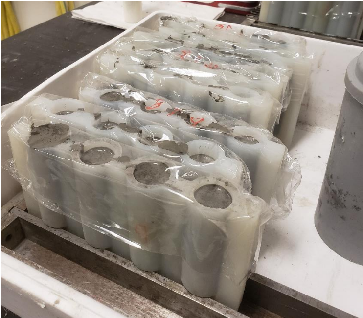
Fig. 4. Silicone molds used to cast binders and mortars in this study
