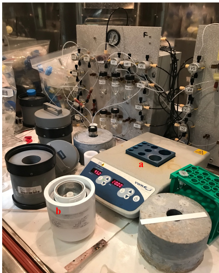
Figure 10 Inside of the hot cell where the radiolabeling was performed, a) heat block, and b) final product collected.
