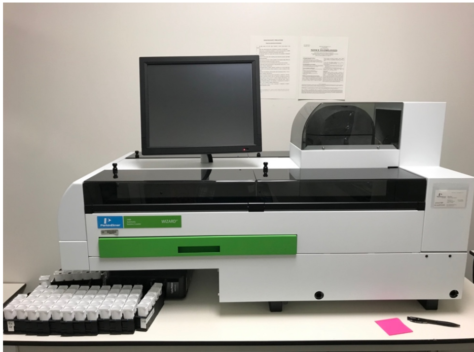
Figure 12 The Perkin Elmer gamma counter used to measure the radioactivity in the tubes.
