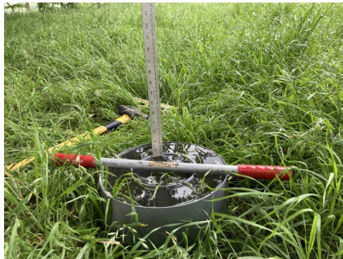
Figure 3.8 SOL_K measurement with double ring infiltrometer at Clear Creek watershed
