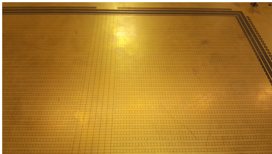
Figure 4.6: A close up picture of the Micromegas plate in TexAT.
