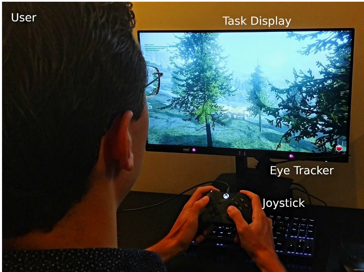
Figure 4.5: Data collection setup used to record human gaze and joystick data illustrating the relative positioning between user, task display, joystick, and eye tracker, as noted in the figure. User is given only the first-person view of quadrotor while performing the visual navigation task.
