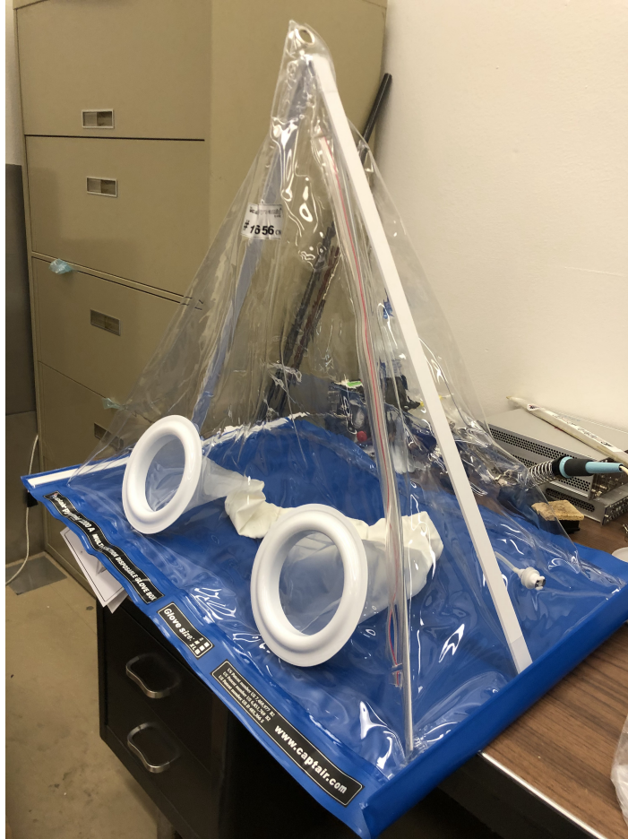
Figure 9.13: An image of the portable glovebag that is essential to the transportation and installation of the target into the beamline and TexCAAM.
