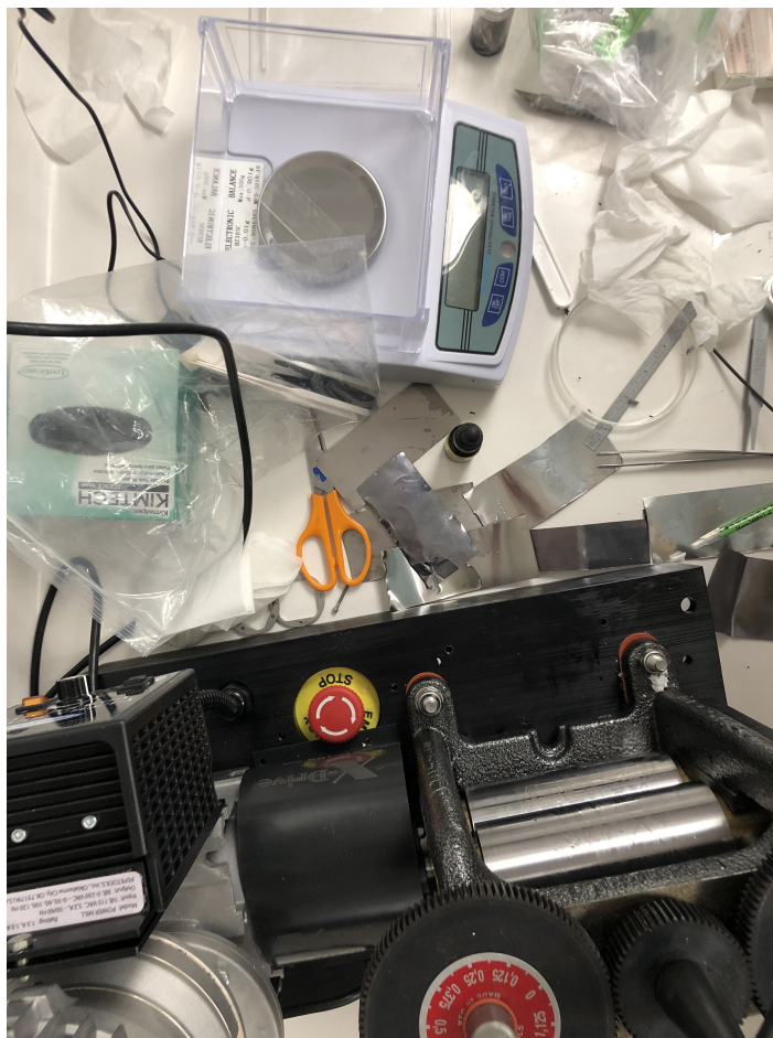
Figure 9.12: An image of the interior of the glovebox. At the top is the scientific scale and at the bottom is the electric metal roller used to create the lithium film target.
