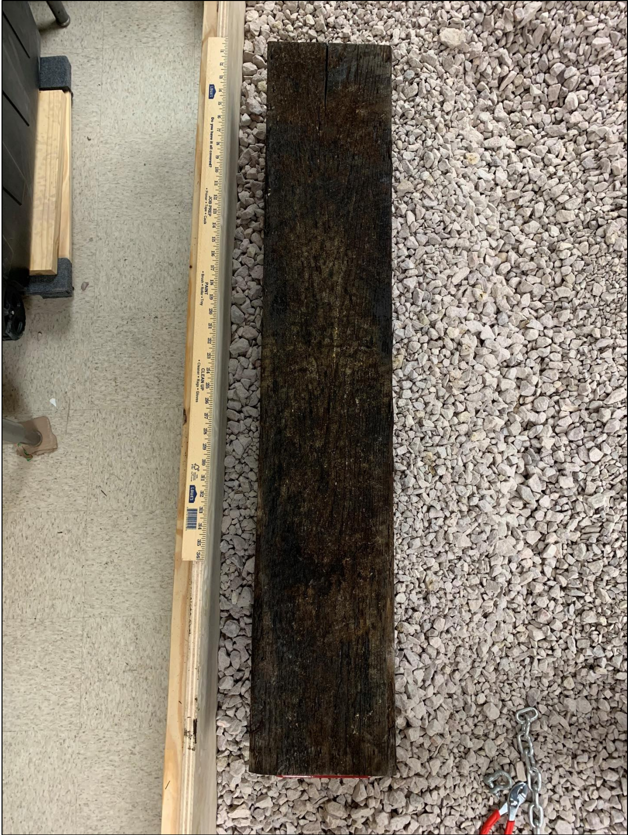
Figure 7: 4 ft cross-tie section
