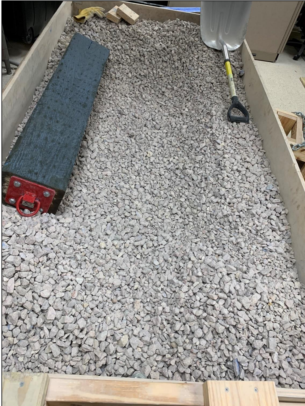
Figure 13: Trench for crosstie alignment
