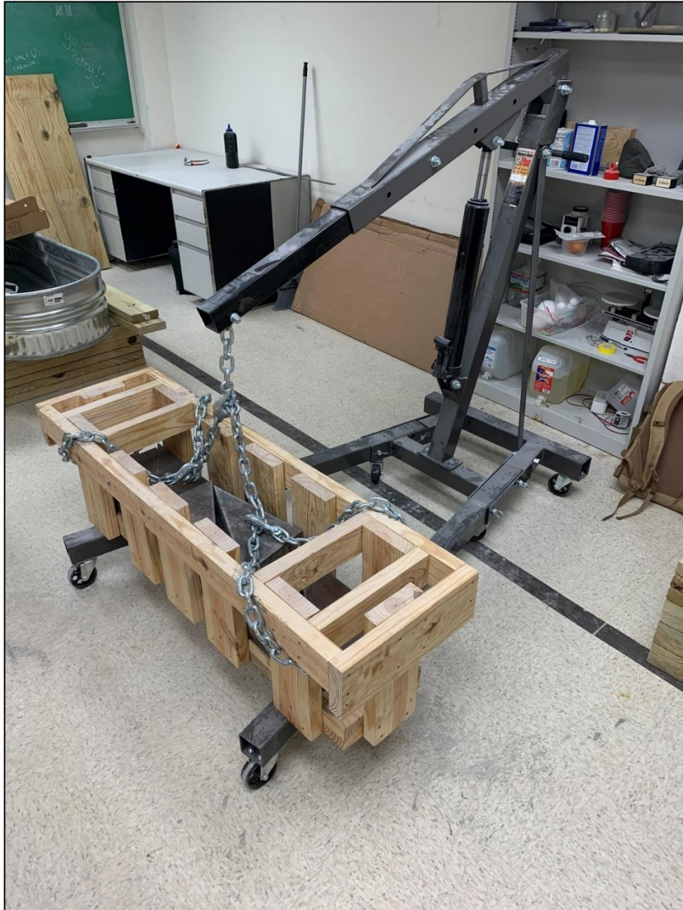
Figure 10: Crane with weight container attached
