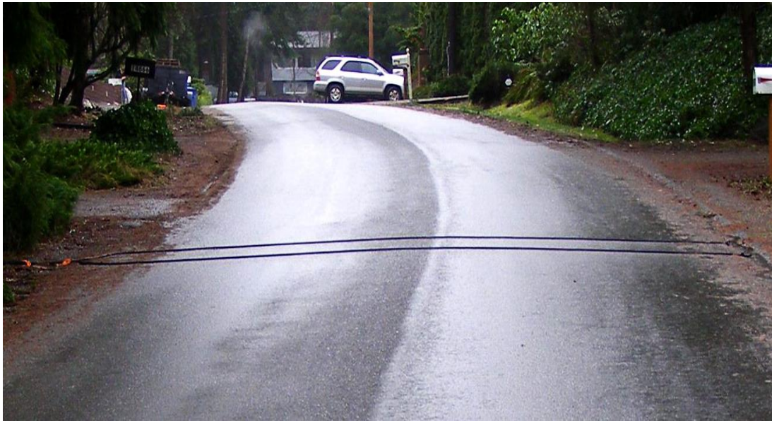
Figure 2: Pneumatic Road Tubes (Reprinted from (Wordpress, 2014))
