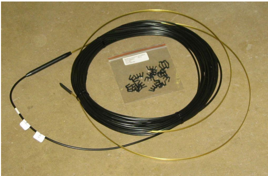
Figure 3: Piezoelectric Sensors (Reprinted from (Counter, 2021))
