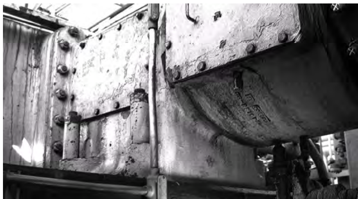
Figure 15: Frame Deflection and Joint Separation MAV
