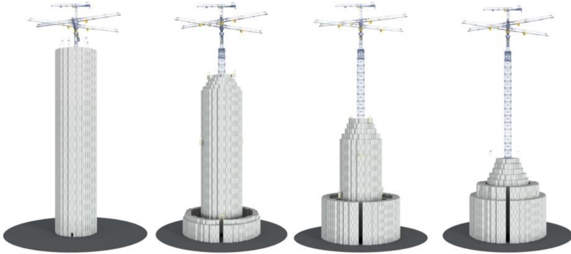
Figure 13. Energy Vault storage tower – higher to lower energy storage from left to right [32]
