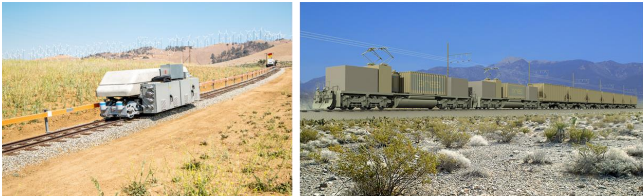
Figure 12. ARES pilot test vehicle (left) and rendering of energy storage rail cars for commercial project in Nevada site (right) [30]
