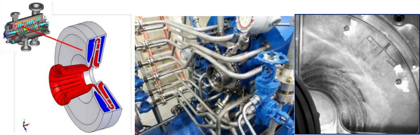
Figure 33. Examples of Advanced Heat Exchange in Turbomachinery: Cooled Diaphragm Concept (left) and Prototype (center) [64]; Air-Water Compression with Direct Cooling (right) [65]
