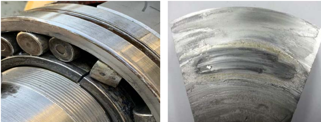
Fig 1 Thrust bearing failures
