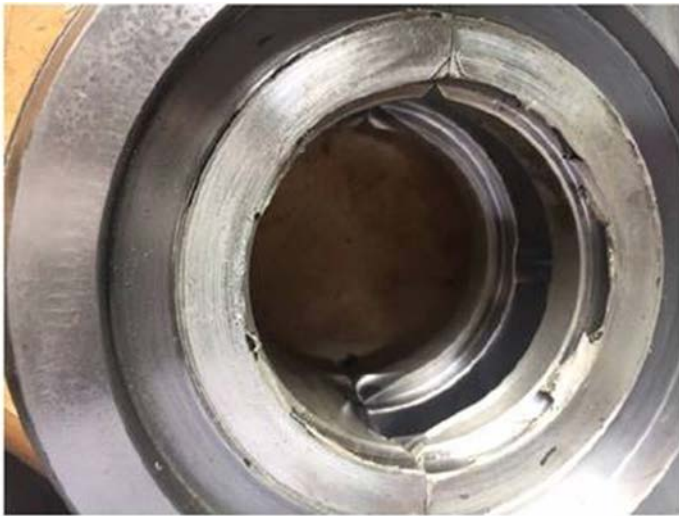
Fig 9 – Rubbing NDE side of Electric Motor
