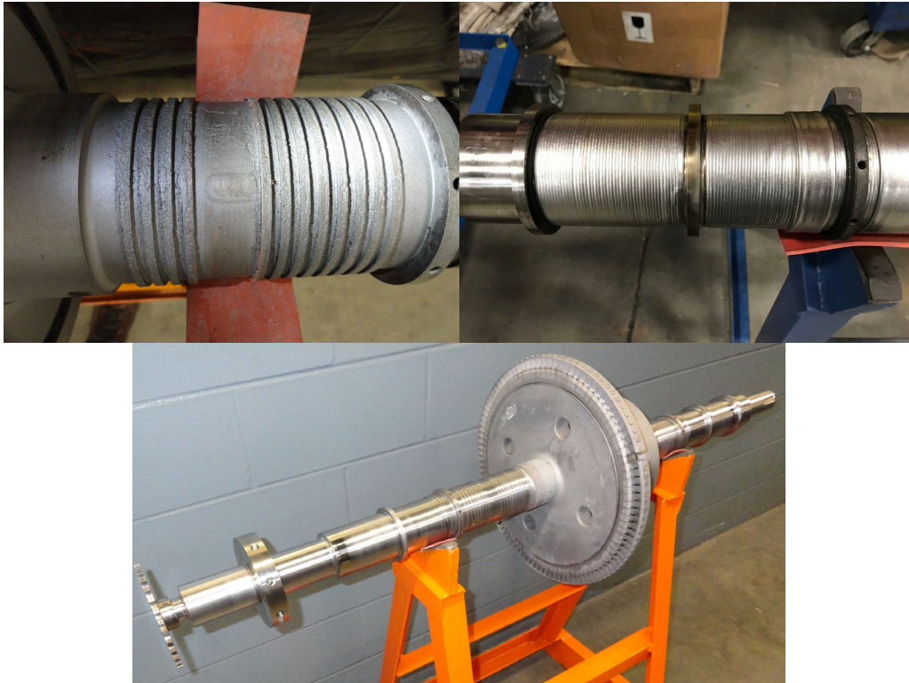
Figure 7: Overlay rotor restoration before repair (top left), after the weld repair (top right) and after final machining (bottom).
