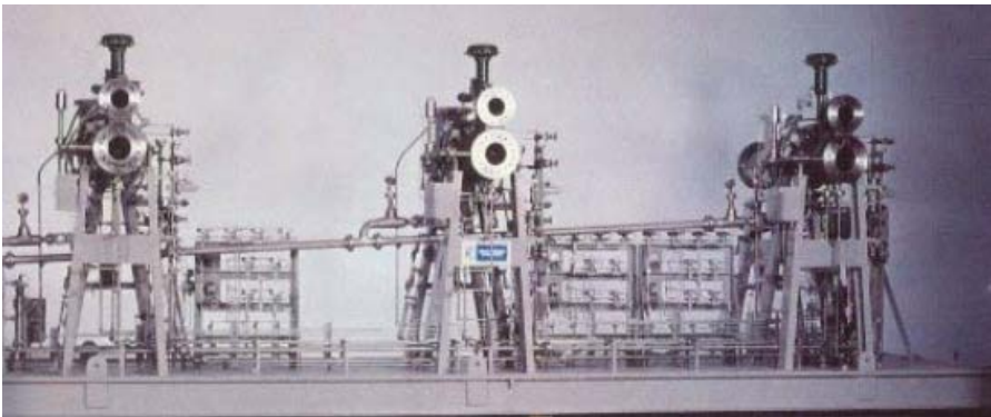
Figure 7. Multi-Stage Expander Compressor with Oil Bearing
