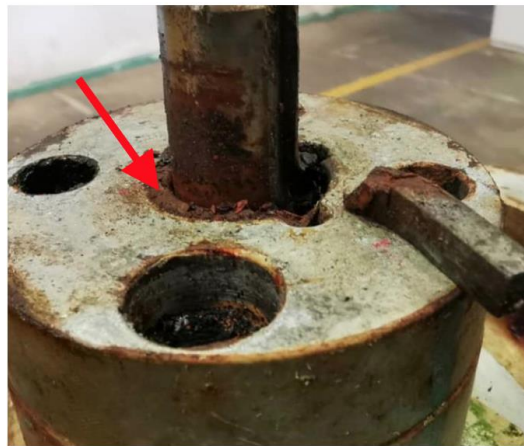
Figure 3 : Anti-surge valve stem dirty due to accumulation of dirt and hardened grease.
