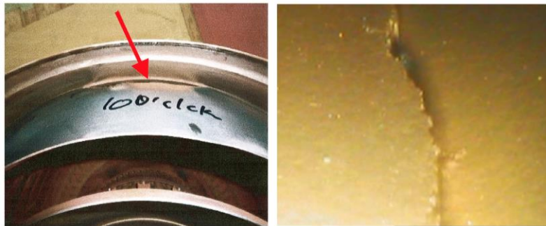
Figure 6: Example of crack happened at stationary combustor hardware resulted from high cycle fatigue
