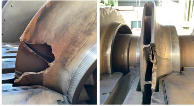
Figure 7: Example of rotor failure at impeller shroud due to diffuser stall.
