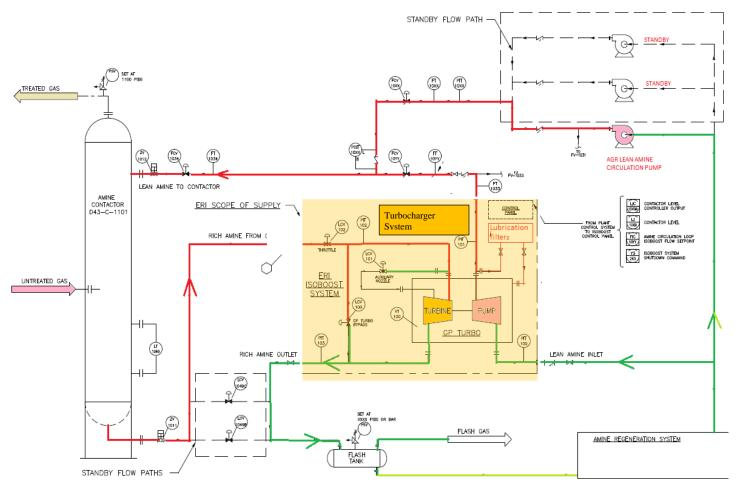
Figure 8: Turbocharger in lieu of contactor level control valve (LCV) and an electrically driven circulation pump
