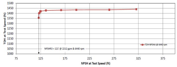
Figure 34: Pump NPSH lab test result
