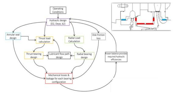
Figure 15: Inter-dependency of Hydraulic and Bearing design
