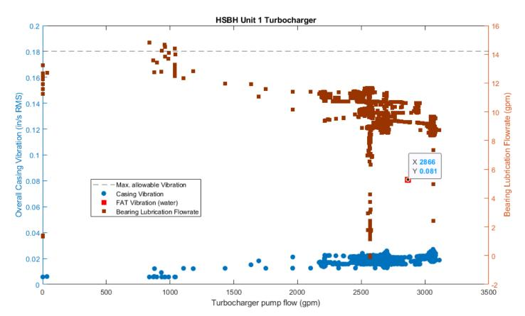
Figure 44: HSBH Unit 1 AGR Plant - turbocharger, casing vibration & bearing lubrication flow rate for October 2020
