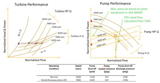
Figure 29: Partial runaway condition for turbocharger (Torque (T) = 0 - runaway condition; Shaft speed (N) = 0 - stalled rotor)25Copyright© 2022 by Turbomachinery Laboratory, Texas A&M Engineering Experiment Station
