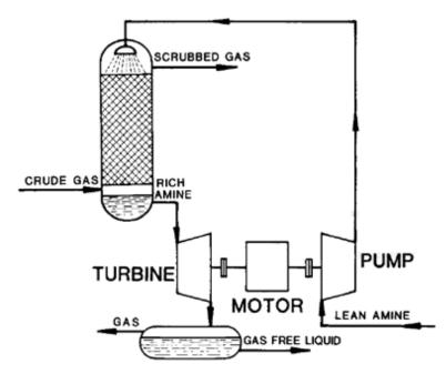
Figure 2: Conventional Pump-Motor-Turbine system (from Gopalkrishnan (1986))
