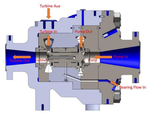
Figure 10: Cross-section of re-designed 3x50% HSBH turbocharger
