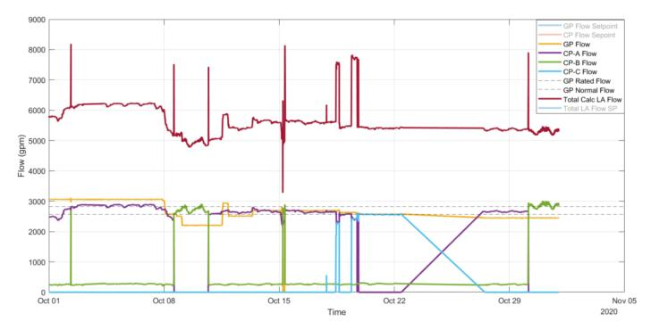
Figure 42: Operational data of turbocharger and circulation pump lean amine flow rates of HSBH Unit 1 AGR plant for Oct 2020
