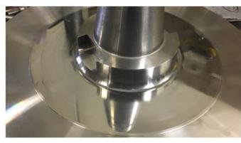
b) Pump back shroud (running face for inactive thrust bearing) in good condition after lab test
