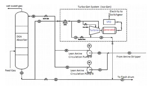
Figure 3: Turbo-Generator generates electricity and feeds it to the grid. Piloted at End User's Hawaiyah Gas Plant.
