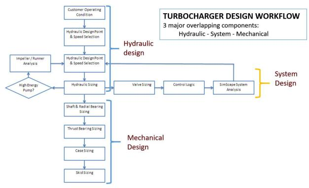
Figure 7: Turbocharger design workflow
