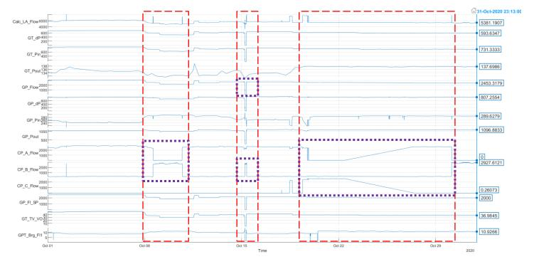
Figure 40: HSBH Unit 1 AGR plant – key operational parameters for the month of October 2020, showing switch-overs between circulation pump and turbocharger
