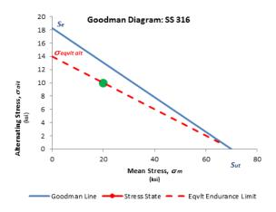
Figure 22: Impeller & runner Goodman diagram
