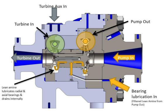
Figure 17: Turbocharger lubrication flow path
