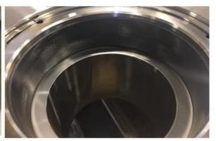
c) Pump wear ring in good condition after lab test
