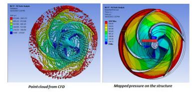
Figure 23: Mapping of hydraulic pressure on impeller walls
