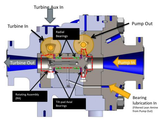
Figure 16: Turbocharger bearing configuration
