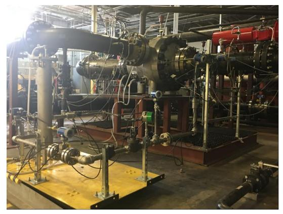
Figure 32: Turbocharger FAT setup with lubrication skid in the foreground
