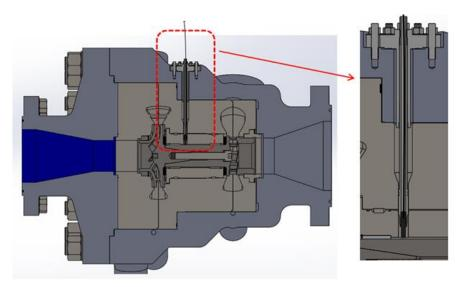
Figure 26: Radial proximity probes
