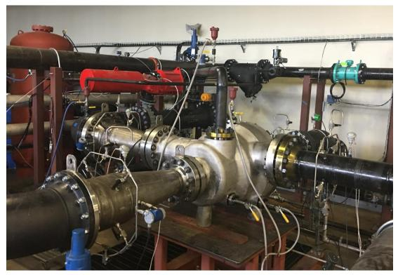
Figure 31: Turbocharger FAT setup showing instrumentation at inlets and outlets of the turbocharger26Copyright© 2022 by Turbomachinery Laboratory, Texas A&M Engineering Experiment Station
