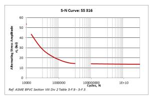
Figure 21: 316SS SN curve for rotating assembly (pump and impeller) fatigue analysis
