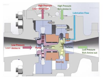
Figure 4: Cross section of hydraulic turbocharger
