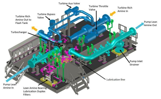
Figure 9: CAD model of turbocharger skid
