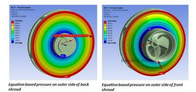
Hydraulic internal Loads on inner side of both the shrouds and blades: (Mapping pressures from CFD)
