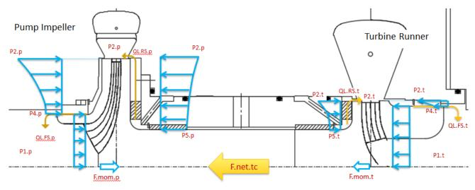
Figure 18: Axial thrust calculation for turbocharger
