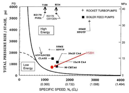
Figure 12: Pump energy level defined in terms of stage pressure rise (from Karassik et al (2000))
