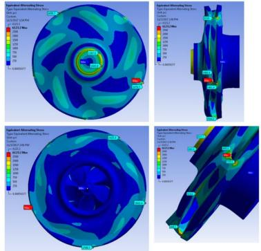
Figure 24: Pump Impeller fatigue FEA analysis
