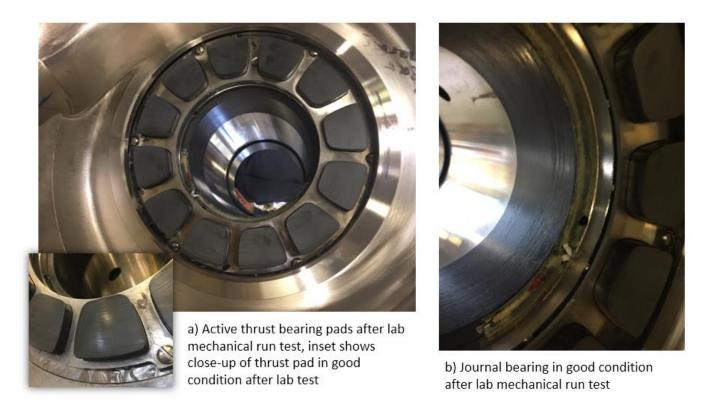
Figure 39: Thrust and journal bearings are in good condition post mechanical run test after bearing rub issue was fixed
