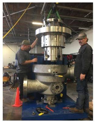
Figure 13: Installation of cartridge in tubocharger casing for FAT
