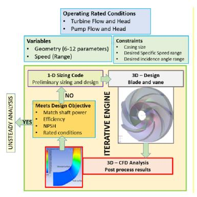
Figure 14: Hydraulic design workflow
