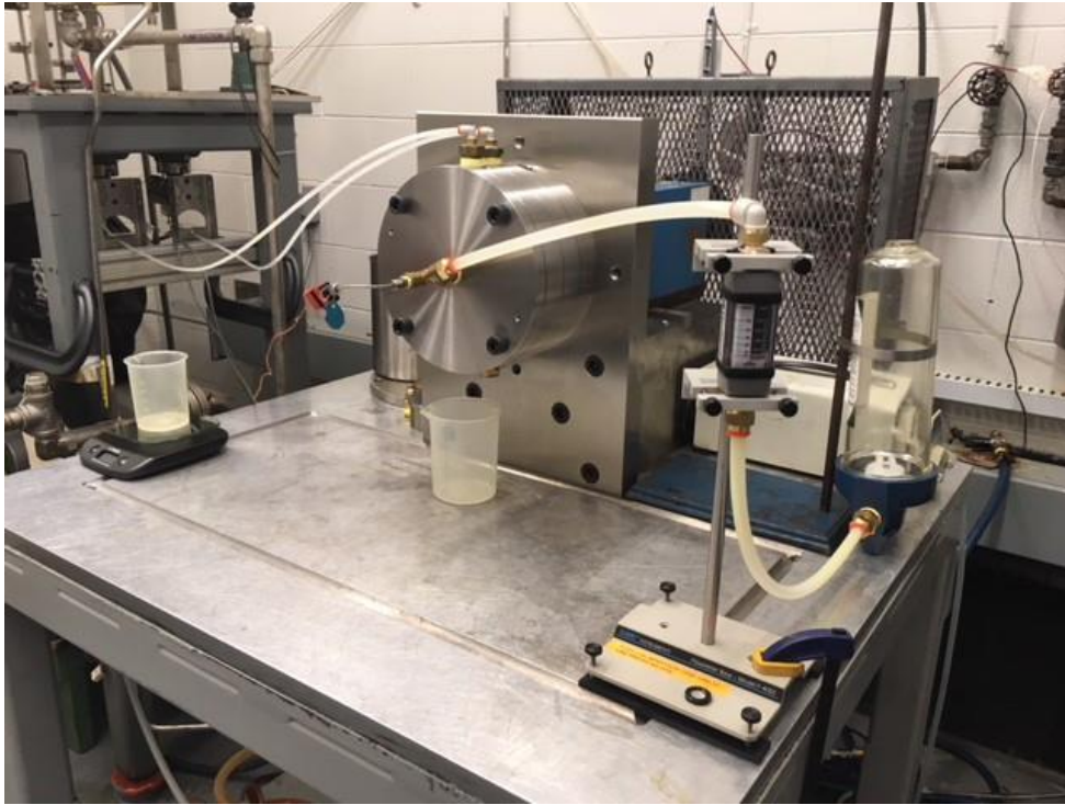
Figure 10 Photo of test rig used for low pressure versus flow investigation of typical bushing
