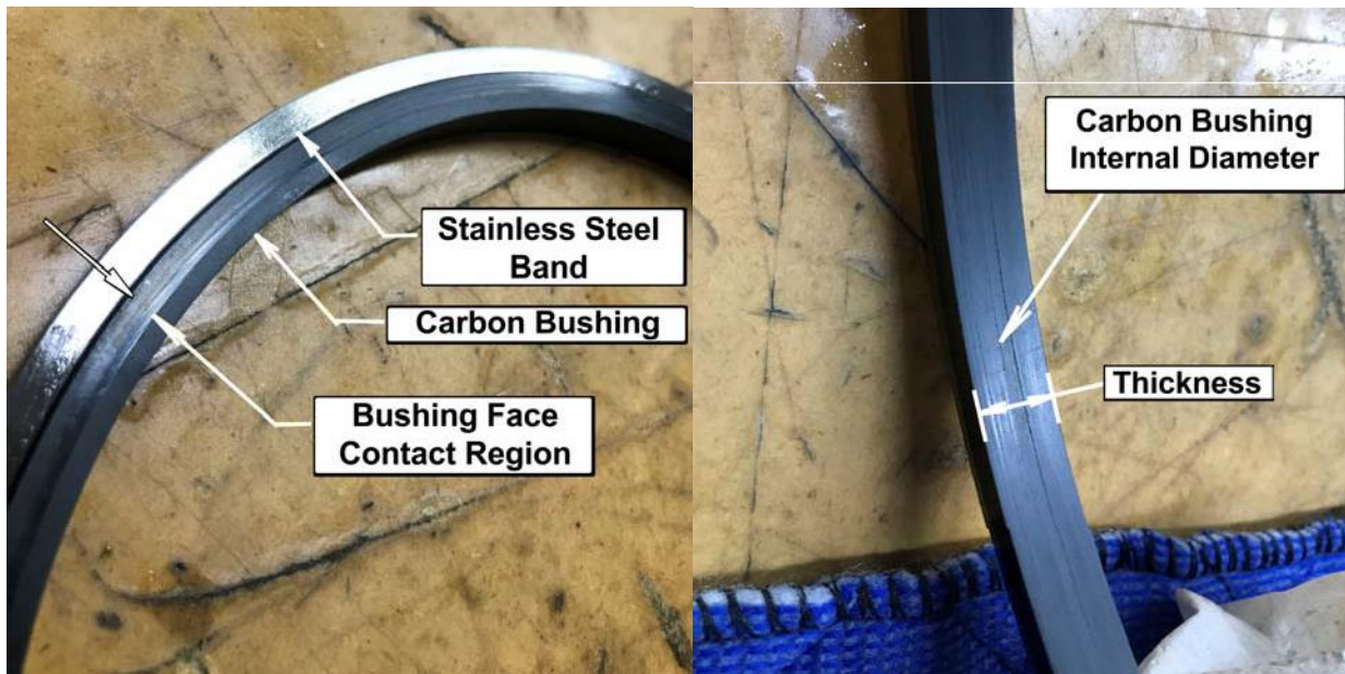
Figure 13 Post catastrophic containment test photos of the primary bushing face and internal diameter
