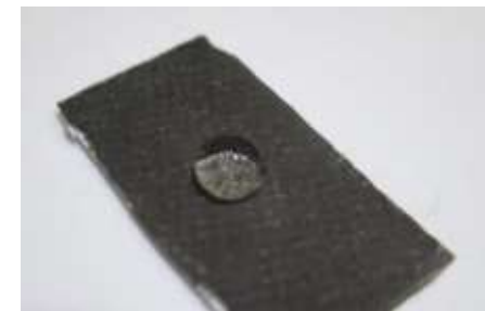
Water repellency test (Upstream Filter Media)
