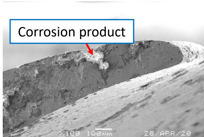
Figure 11: Blade 1 Separation Surface
