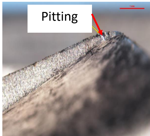
Figure 5: Blade 1 Separation Surface at Leading Edge
