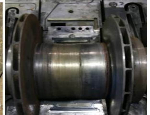
3 rd & 4 th stage compressor centre seal (honey comb) badly rubbed & sleeve materials loss
