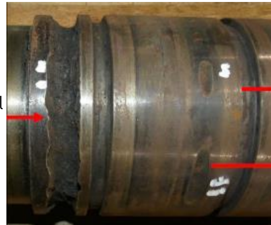
3 rd & 4 th stage compressor centre seal (honey comb) badly rubbed & sleeve materials loss
