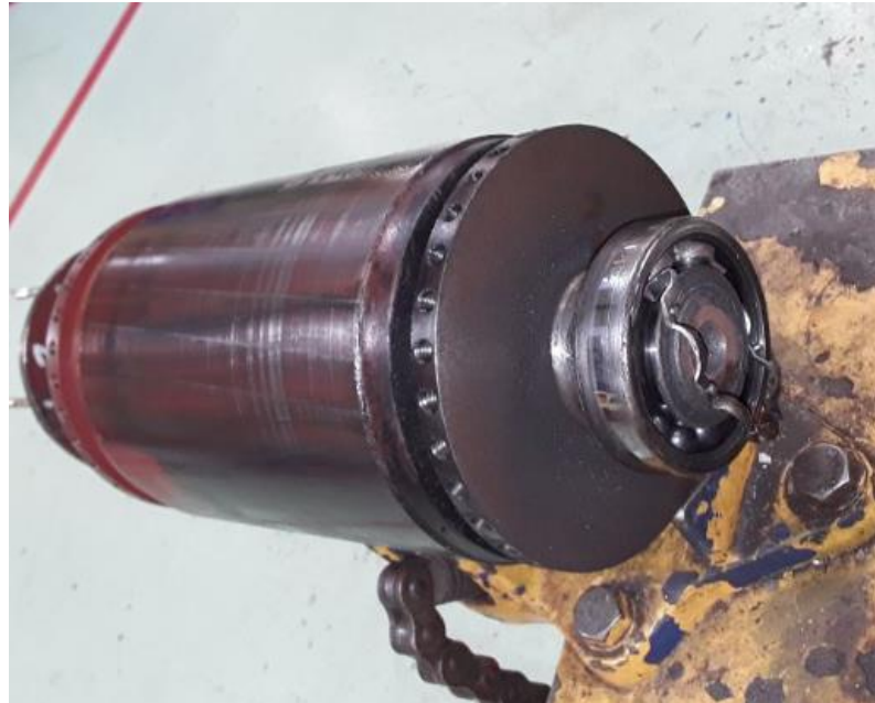
Figure 5: Turning Gear Motor as found damaged on May 24, 2020; NDE bearing was found collapsed
