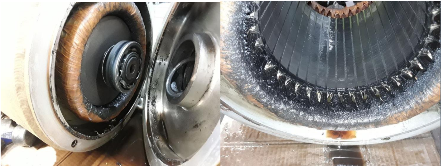
Figure 6: Turning Gear Motor as found damaged on May 24, 2020; The signs of oil in the stator windings and endshields.
