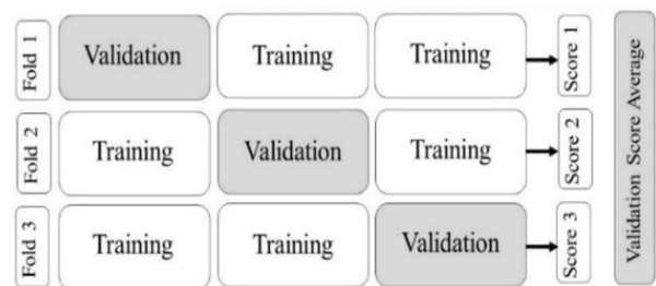
Figure 2 The K-fold cross-validation method, where the average of the three resulted scores are considered to evaluate the NN model
