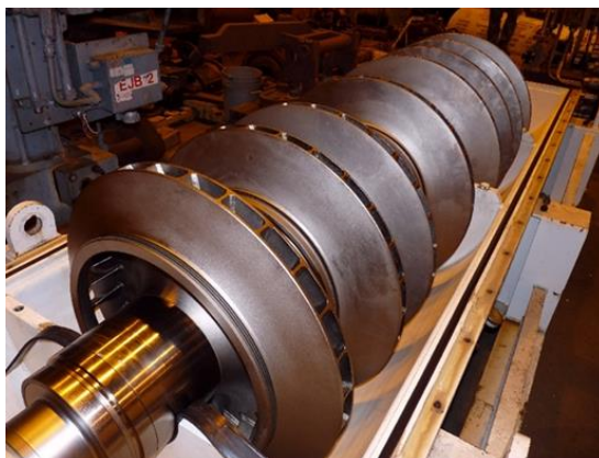
Figure 30: Compressor Rotor with Electroless Nickel Coating
