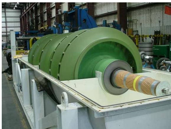
Figure 29: Compressor Rotor with a PTFE Topcoat
