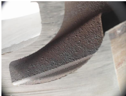
Figure 28: Pitting Corrosion in 17-4 PH Stainless Steel Underneath Foulant Build-up in Figure 27
