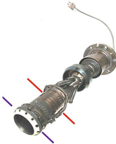
Figure 6: Burner repairs in the traditional fashion (red line) and the described novel repair process (purple line)
