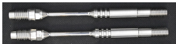
Figure 2. Proof ring specimens for hydrogen tests
