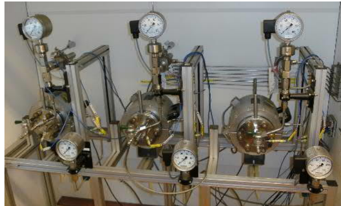
Figure 7. Heated test pressure vessels (autoclaves)
