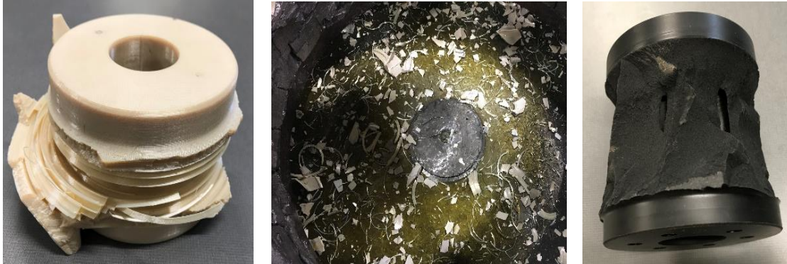
Figure 7 – Impeller after destructive testing
