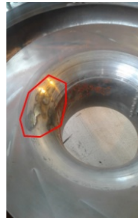
damaged 2 nd stage casing
