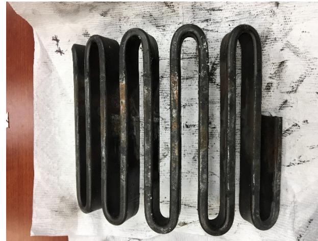
Broken Grid Coupling Element + Indications of Excessive Heat
