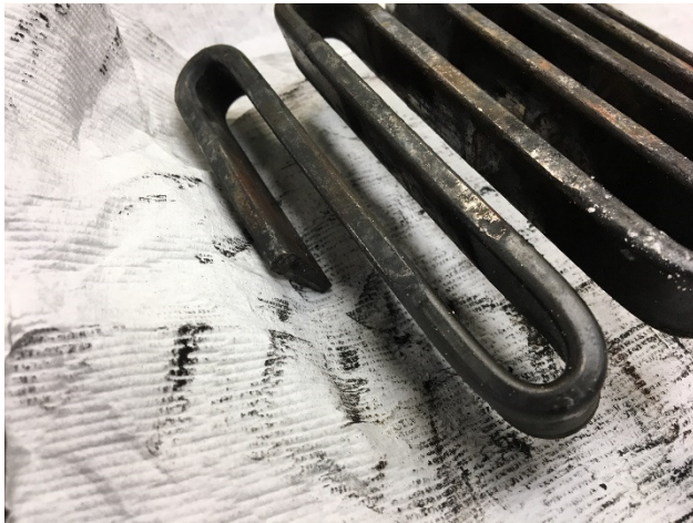
Broken Grid Coupling Element + Indications of Excessive Heat
