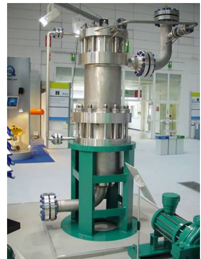
Figure 6 Vertical canned motor pumps to reduced radial load of rotor
