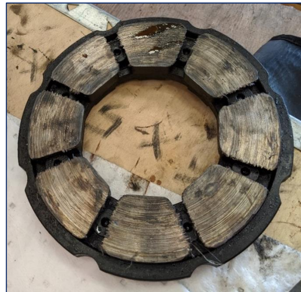
Damaged Thrust Bearing and Trending before the Failure
