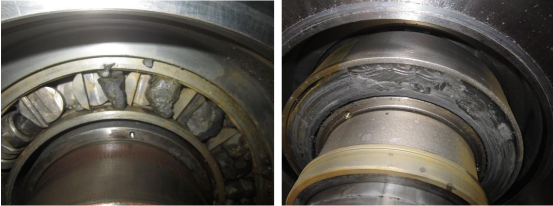
Figure 2: A failed product lubricated ceramic TPTB.
