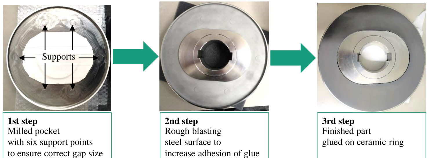
Figure 16: Thrust collar assembly process
