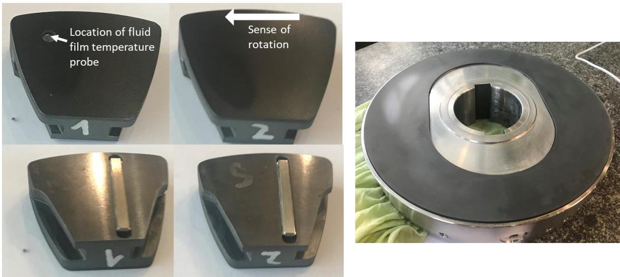
Figure 23: Post-test condition of the pads and thrust collar in ceramic TPTB after a 36 hour test campaign.
