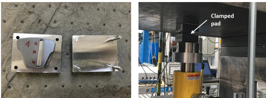
Figure 13: (a) pad and clamp, (b) load application on pad with a hydraulic press.
