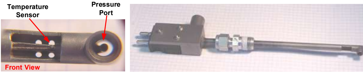
Figure 23: Combination total pressure/total temperature probe used for flange-to-flange measurements.
