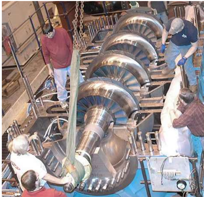
Figure 15 – Rotor being installed in bottom half of a horizontally-split compressor
