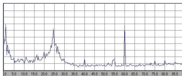
Figure 41. Peak hold vibration spectrum - arbitrary aerodynamic forces.
