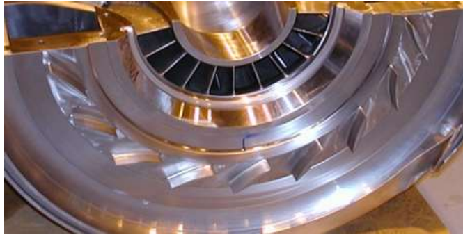
Figure 23. Low solidity diffuser vanes (LSDs)
