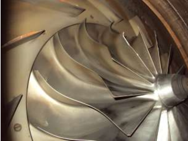
Figure 17: First Stage Blade Failure
