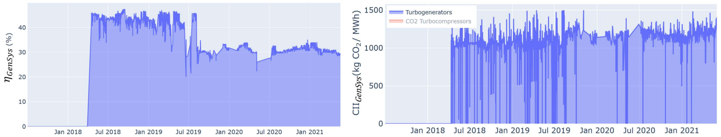
Figure 10. Overall Efficiency and Carbon Intensity Index Associated to the Main Power Generation System
