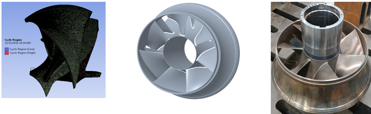
Figure 11. FEA, Solid Model and Test Impeller
