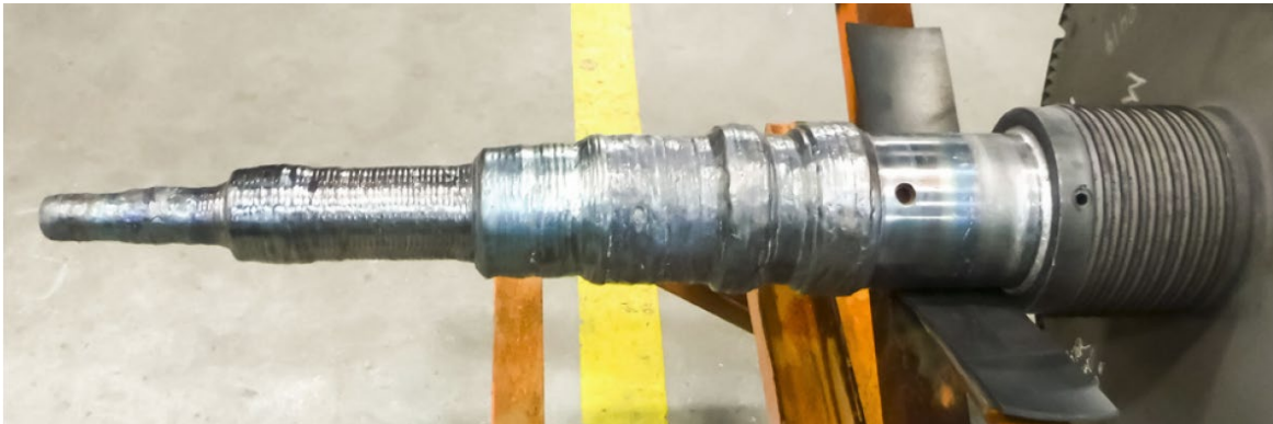
Figure 1: An example of a SAW repair on a rotor. Note the large surface area requiring overlay, much of which was added to ensure the rotor would have enough machining stock to account for distortion induced by the repair process.
