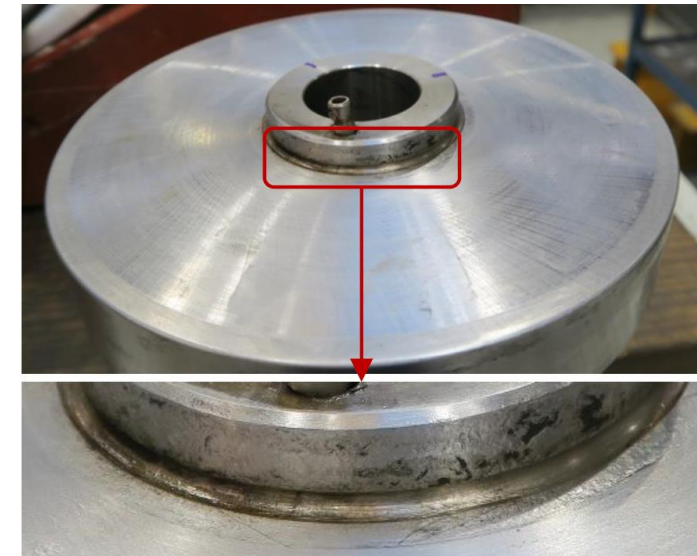
Figure 11 – Damaged Thrust Collar
